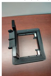
This is the final version of the 3D printed electrical box that the SiMT Manufacturing team was able to fabricate.
