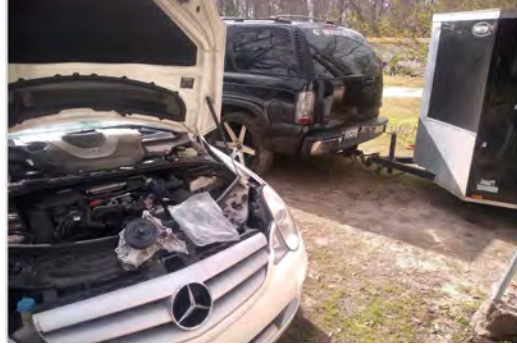
R Class Mercedes Benz with coolant leaks. Get a pressure test done to go to the problem. Water pump replacement done at clients home. Well below dealership cost.
