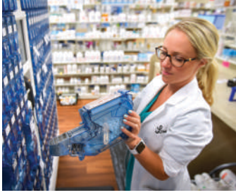
Jess Kemmler, PharmD, checks the supply of pills in the Parata Max automated robotic dispenser. The Parata Max is designed to help pharmacies efficiently label, count, sort, and cap prescriptions. Dr. Kemmler is a pharmacist at Long's Drugs located inside the HopeHealth Medical Plaza in Florence.
